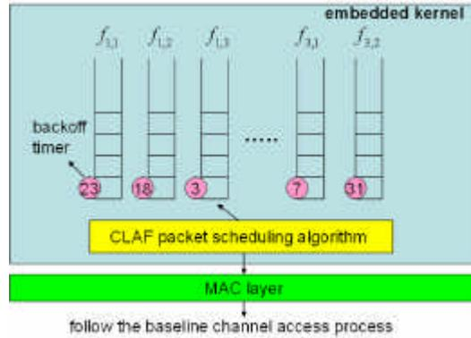
Fig. 3. The implementation architecture of the packet scheduling and queuing at a wireless station in the CLAP service model
