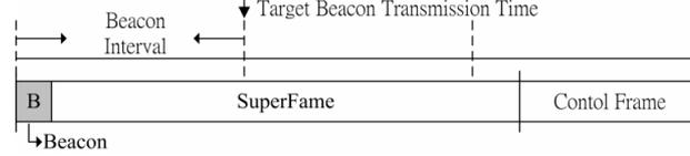
**Fig. 5.** A channel access round consists of a superframe for multi-class packet transfer plus a control frame for notifying flow join and leave
